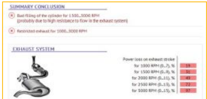
Figure 10: Severe exhaust system restriction.
