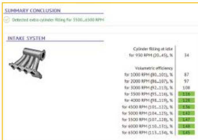
Figure 8: Summary conclusion on volumetric efficiency on a turbocharged engine.
