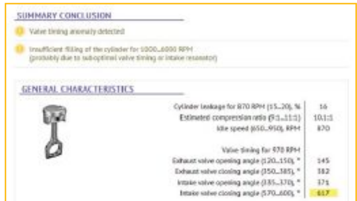
Figure 5: Summary conclusion on an engine with late valve timing.
