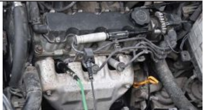
Figure 1: Pressure and synchronization transducer installation.
