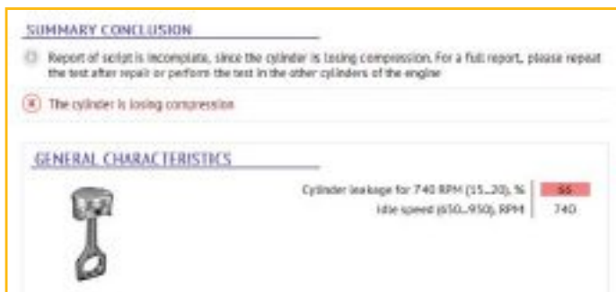
Figure 3: Audi engine with compression loss.
