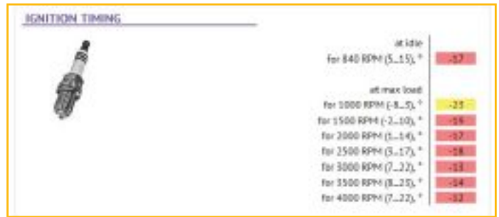
Figure 12: Summary conclusion showing late ignition timing at various rpm ranges.
