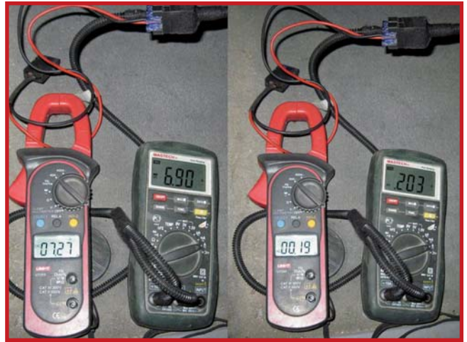
Figure 4: Measuring AC and DC current on a fuel pump circuit.
