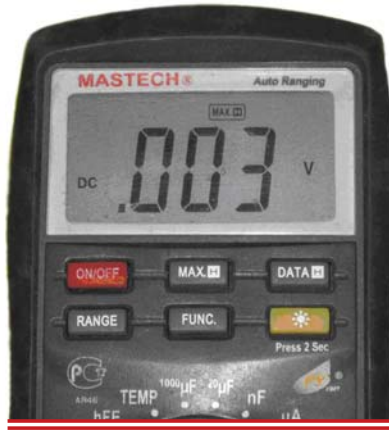
Figure 6: A DMM showing the max hold mode being used.
