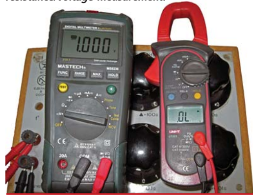
Figures 4a and 4b: Comparing diode test and resistance/voltage measurement.
