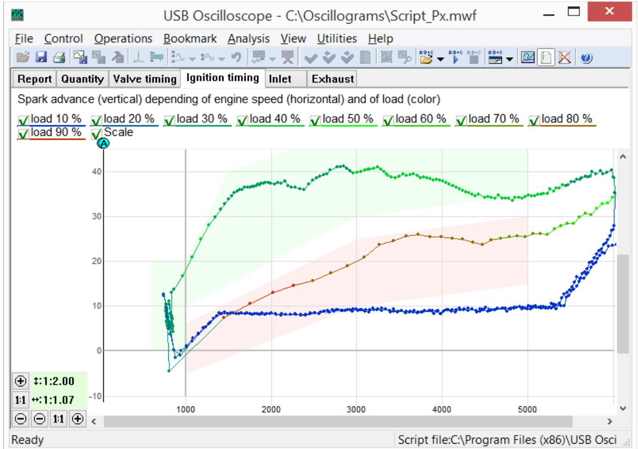
*Typical diagram from the "Ignition timing" tab. This engine is in good operating condition. Here the low load or overrun trace is activated.*
