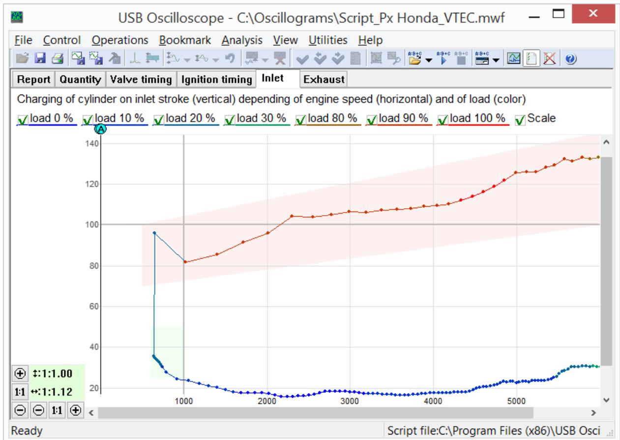
*Cylinder filling diagram from an engine with a 4 valves per cylinder and a different induction system design.*
