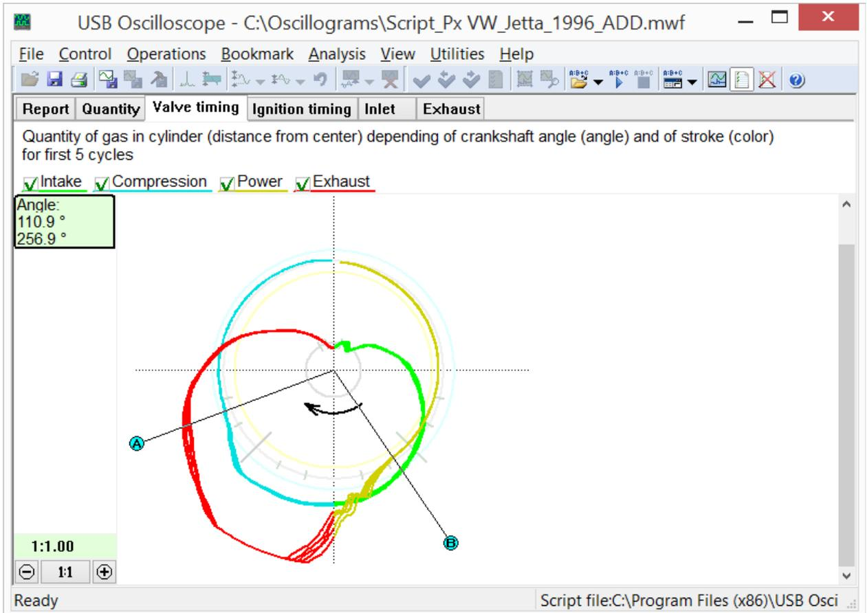
*Polar diagram from an engine with late valve timing. The valves are opening and closing late. The A marker shows where the intake valve is closed, and the B marker shows where the exhaust valve starts to open.*
