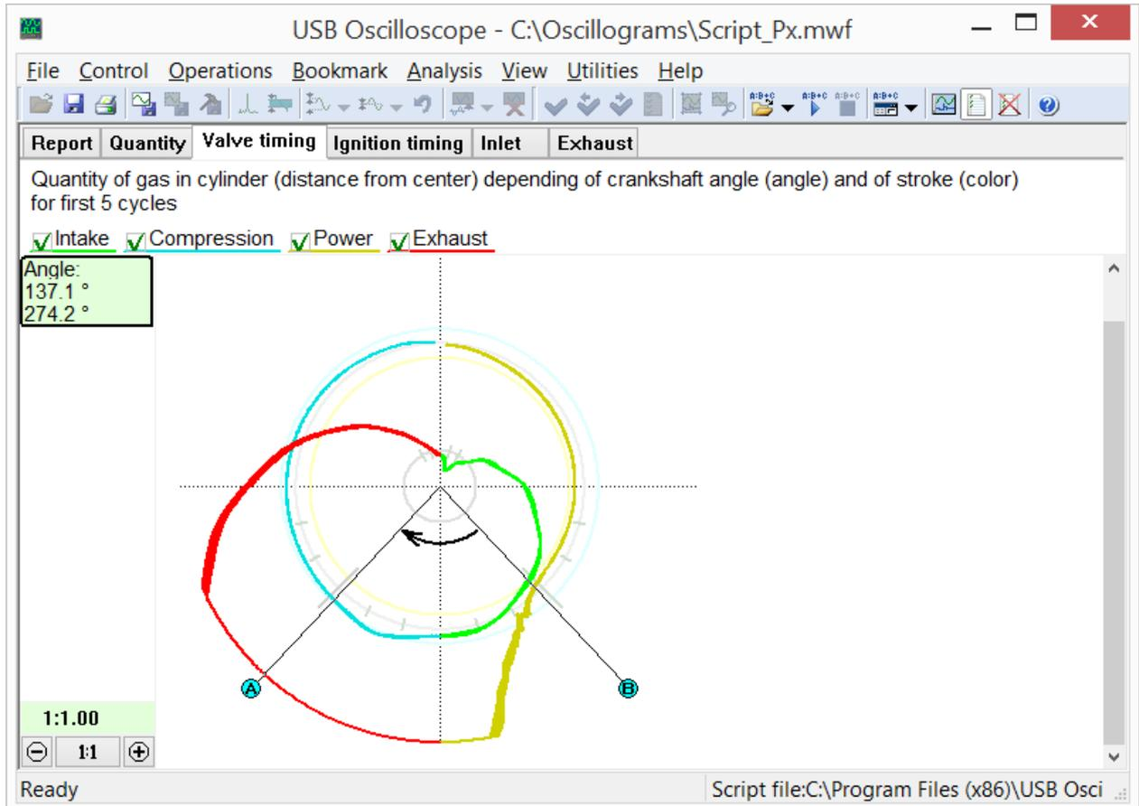
Typical diagram from the "Valve timing" tab. This is an engine in good working order. This diagram shows the amount of gas in the cylinder depending on the angle of the crankshaft and the stroke of the tested cylinder. The A marker shows where the intake valve is closed, and the B marker shows when the exhaust valve begins to open. Note that the marker locations are symmetrical relative to the vertical line.
