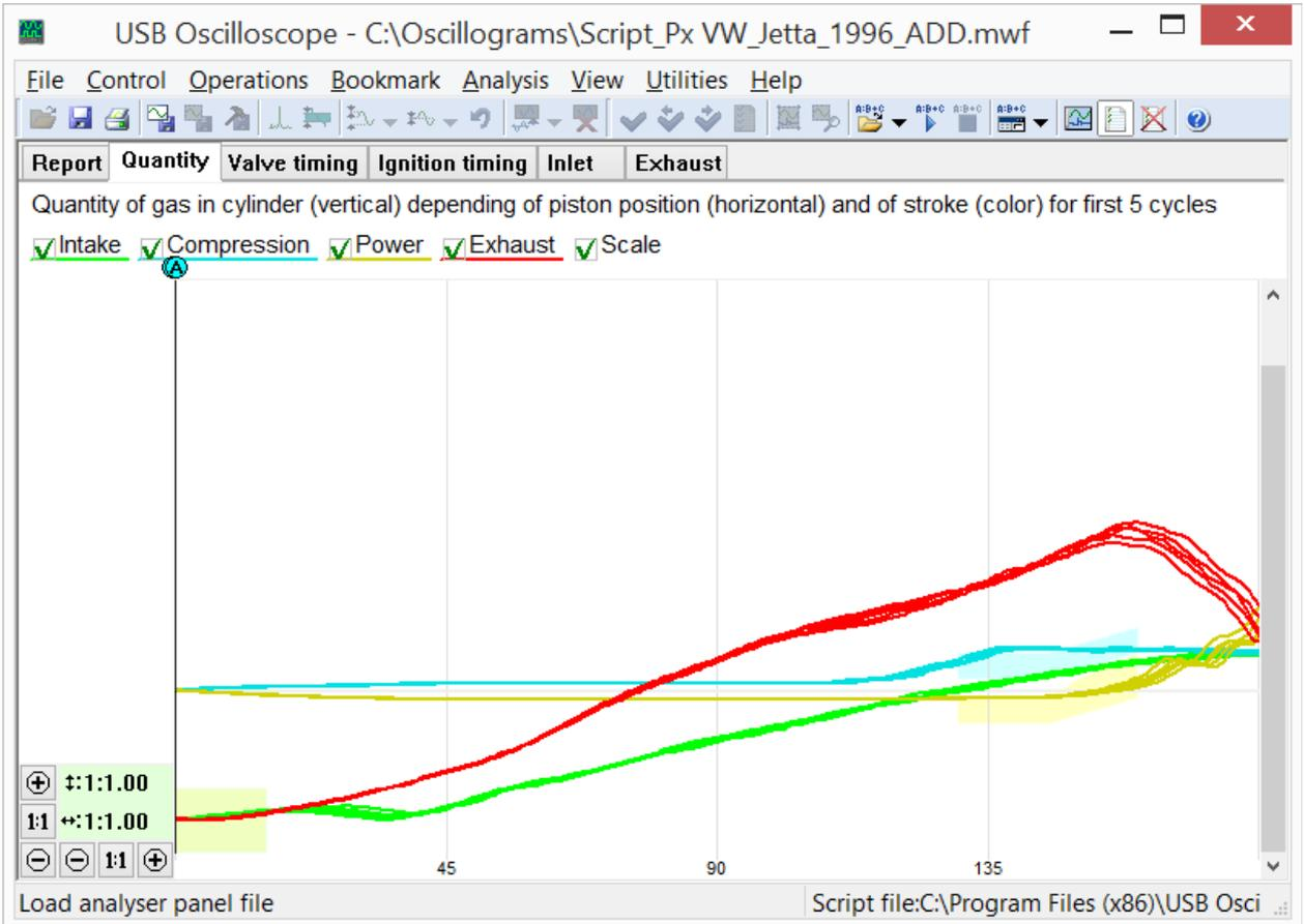
*Valve timing is set incorrectly so the valves open and close late.*
