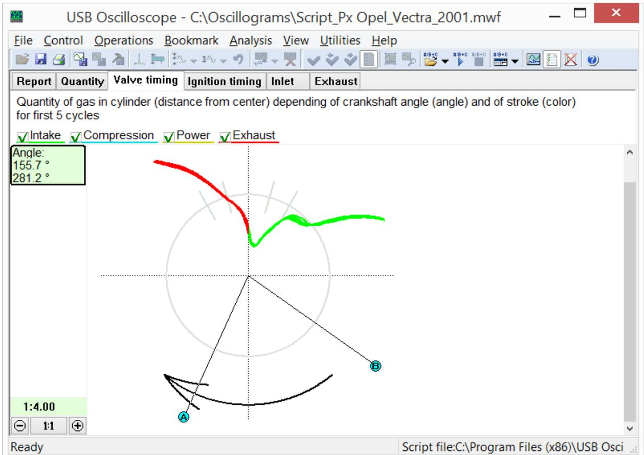
*This zoomed figure shows the distortion of the timing diagram in the center, due to the early or advanced valve timing.*
