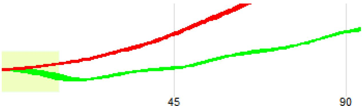
This is the characteristic shape of the left part of the red and green traces from an engine in good condition.
