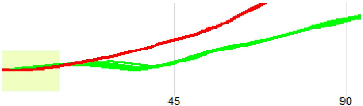
*In this figure, can be seen that the red and green traces displaying the amount of gas in the cylinder are superimposed on each other for the first part of the crankshaft rotation.*
