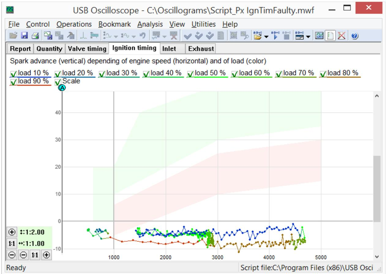
*This is a timing diagram showing abnormal timing control.*
