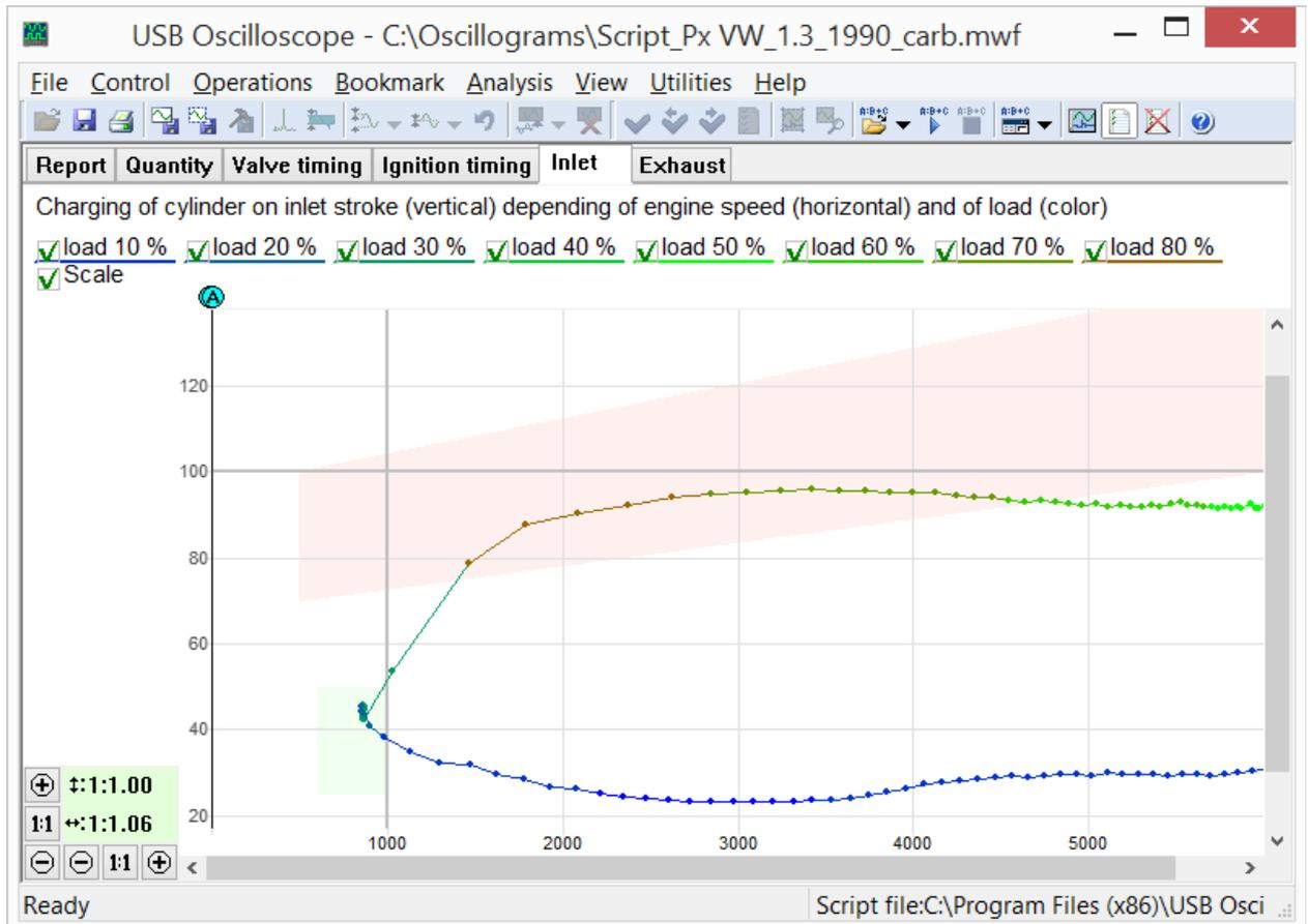
*Cylinder filling diagram from an engine equipped with a carburetor and one intake and one exhaust valve per cylinder.*
