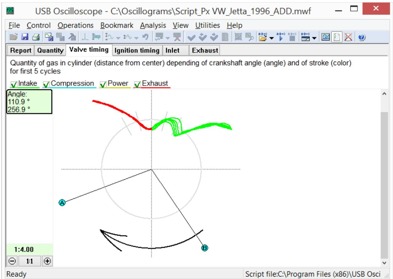
*Typical distortion of the valve timing diagram in the zoomed center. The distortion is due to late valve timing.*
