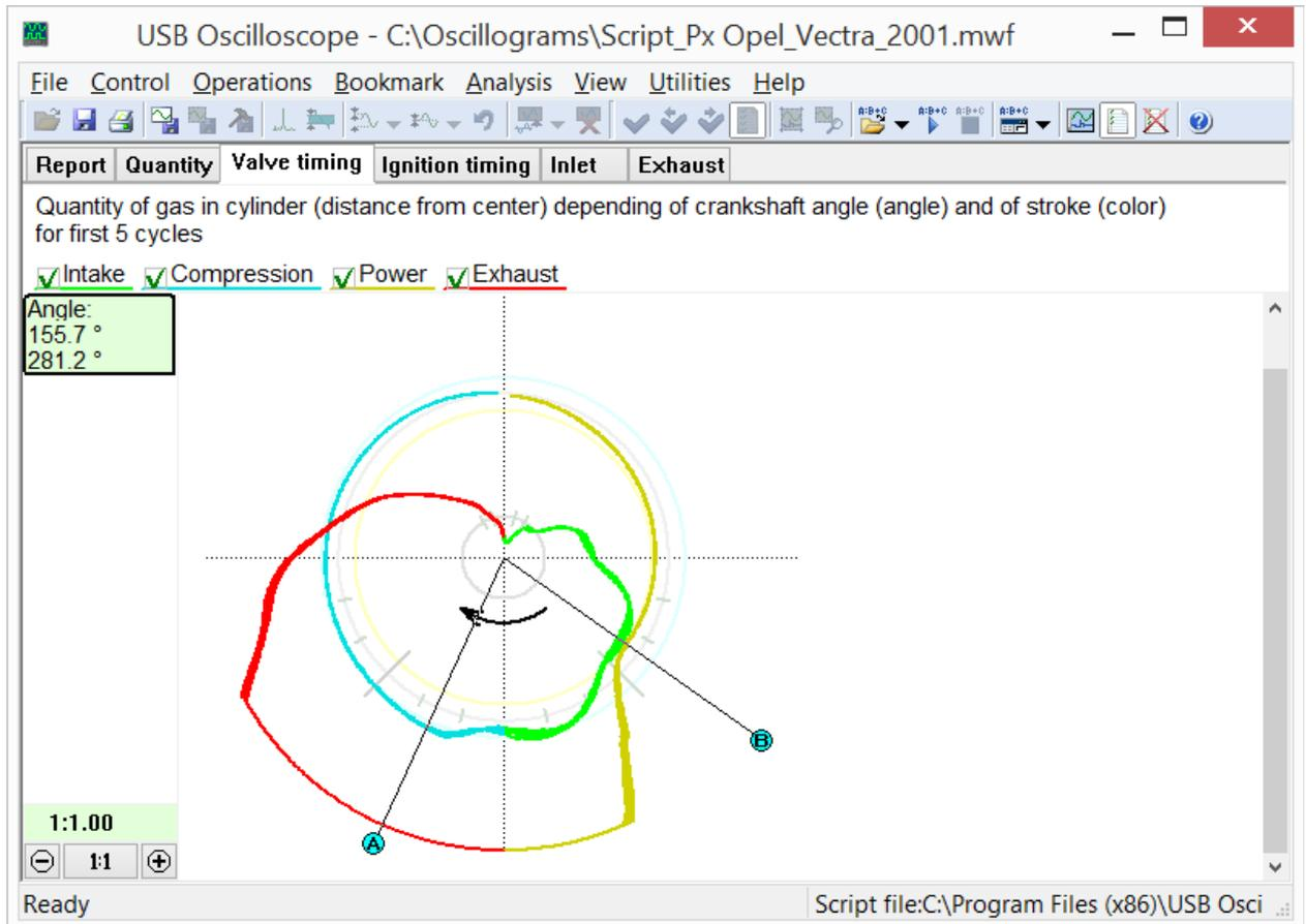
*The valve timing phases are asymmetrical showing an incorrect valve timing. In this example the cam timing is advanced one tooth. The A marker shows the angle when the intake valve is closed, and the B marker shows when the exhaust valve started to open.*
