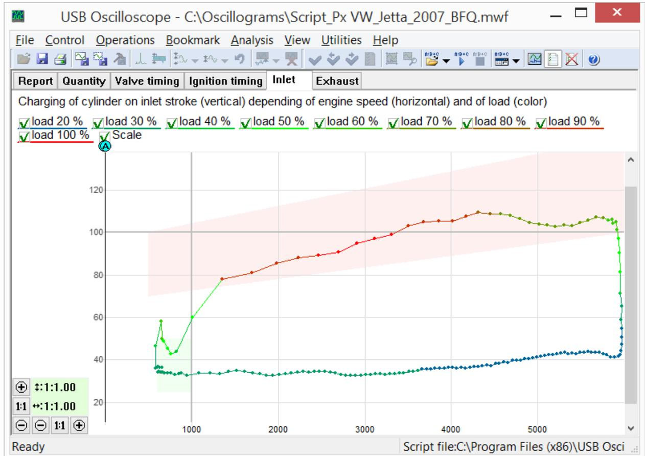
*This graph from the Inlet tab was recorded using two throttle snaps, fast and slow.*
