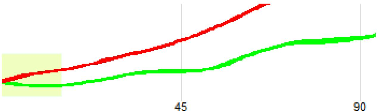
*Typical waveform distortion seen when the valve timing is advanced.*
