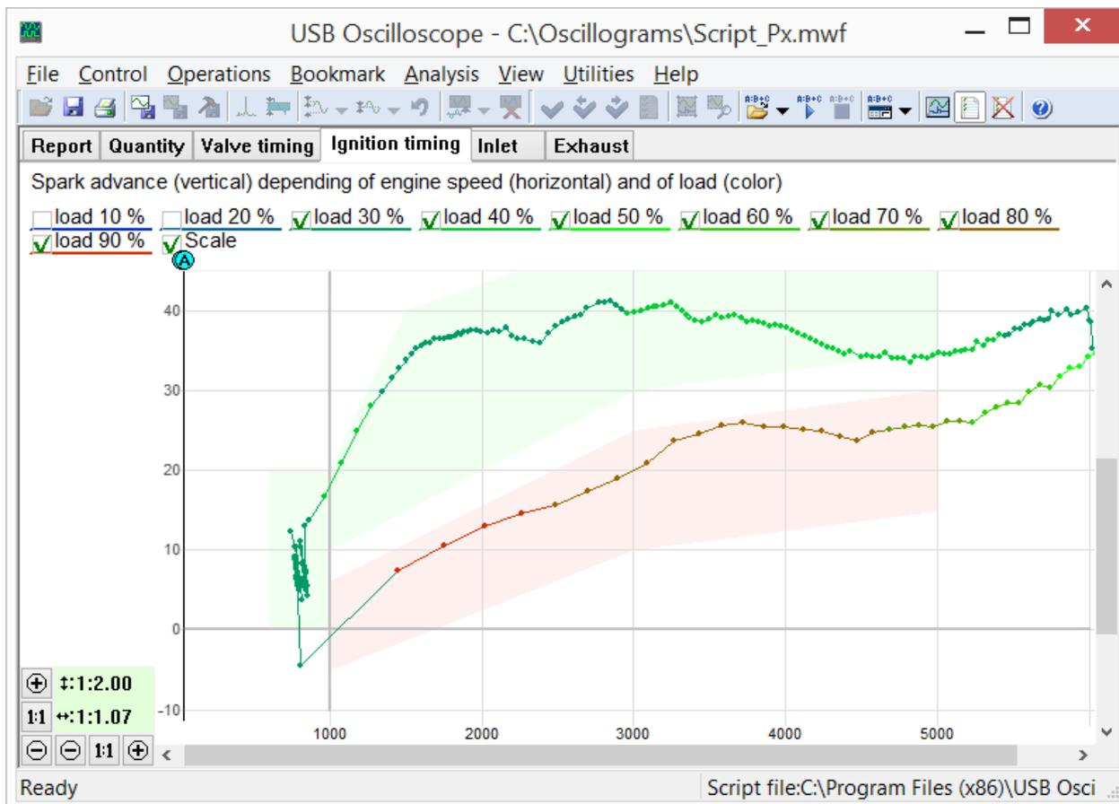
*This is an ignition timing diagram from an engine in good working order. The data is taken from two throttle openings. One sharp and one smooth opening.*
