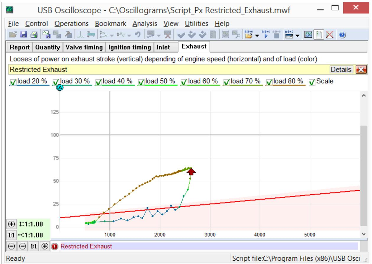
*This diagram shows a fairly severe exhaust system restriction. In this case the problem was a plugged catalytic converter.*
