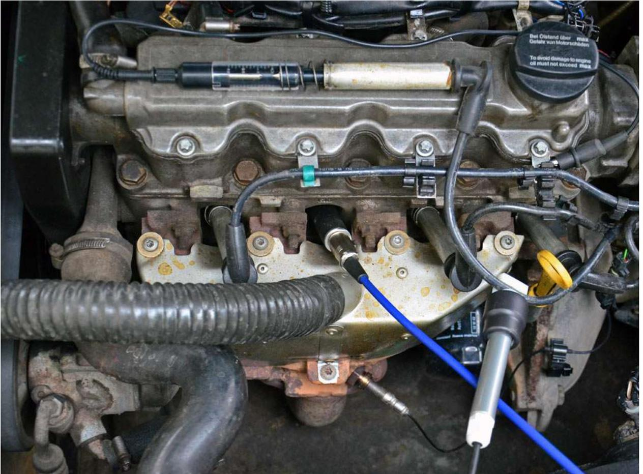
*The pressure transducer replaces the spark plug.*
