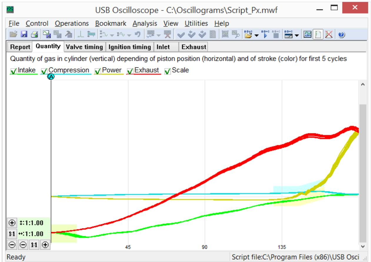
The "Quantity" tab from the Px script report, this engine is in good condition. The graph indicates the amount of gas in the cylinder relative to the position of the piston in the cylinder and the stroke.
