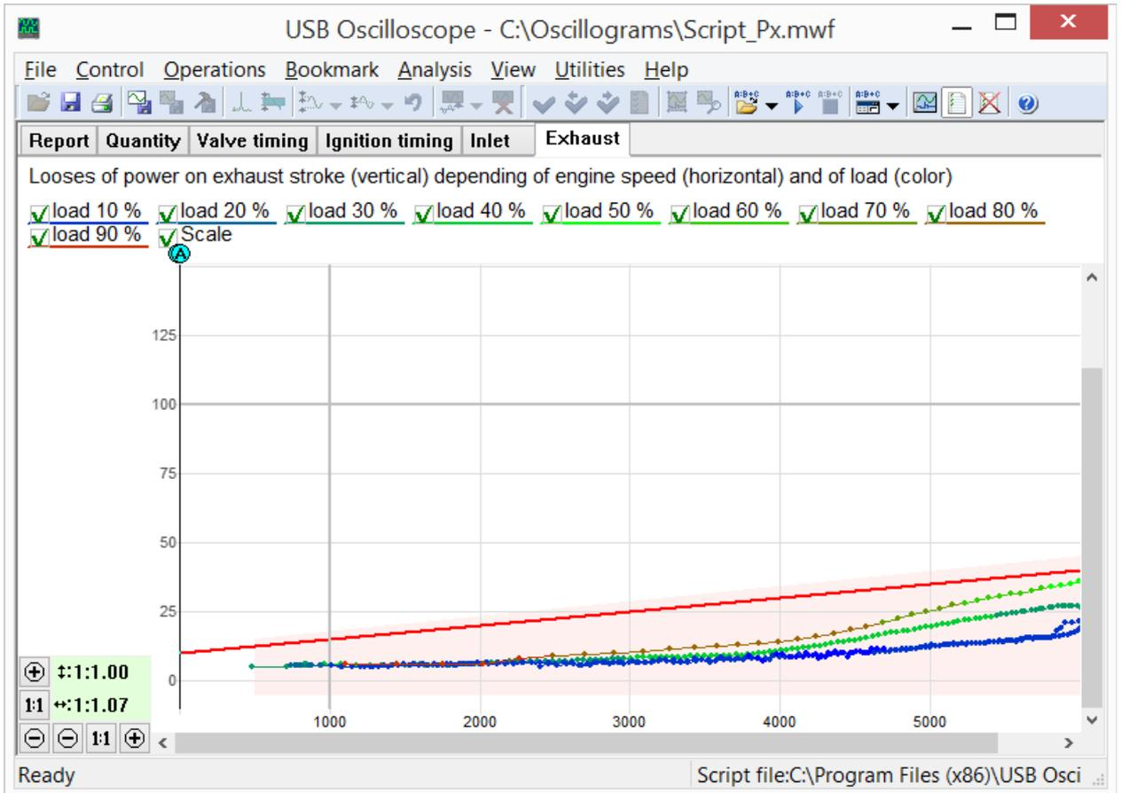
*The "Exhaust" tab. This diagram taken from an engine with normal exhaust system restriction.*
