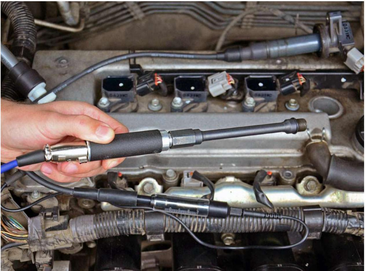
*If the spark plugs are recessed, necessitating using an extension, a deep well adapter should be used.*
