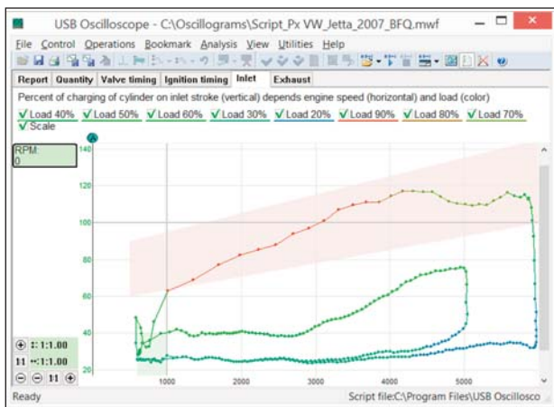
Figure 1: This graph from the Inlet (or Intake) tab was recorded using two throttle snaps, fast and slow. This is an engine utilizing a throttle for rpm control.
