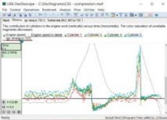
Figure 3: Efficiency tab from a 2014 Chevrolet Aveo.
