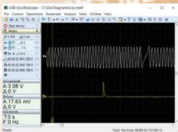
Figure 2: CKP and ignition signal as shown on an oscilloscope screen.
