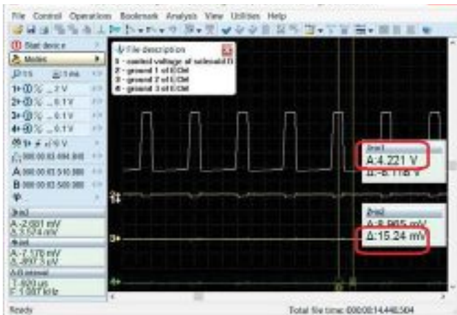
Figure 5: Ground circuit waveforms along with the low or ground circuit for the pressure control solenoid.
